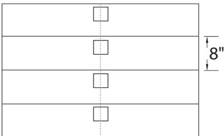
Mount in center of stair as close to the upper tread as possible.
